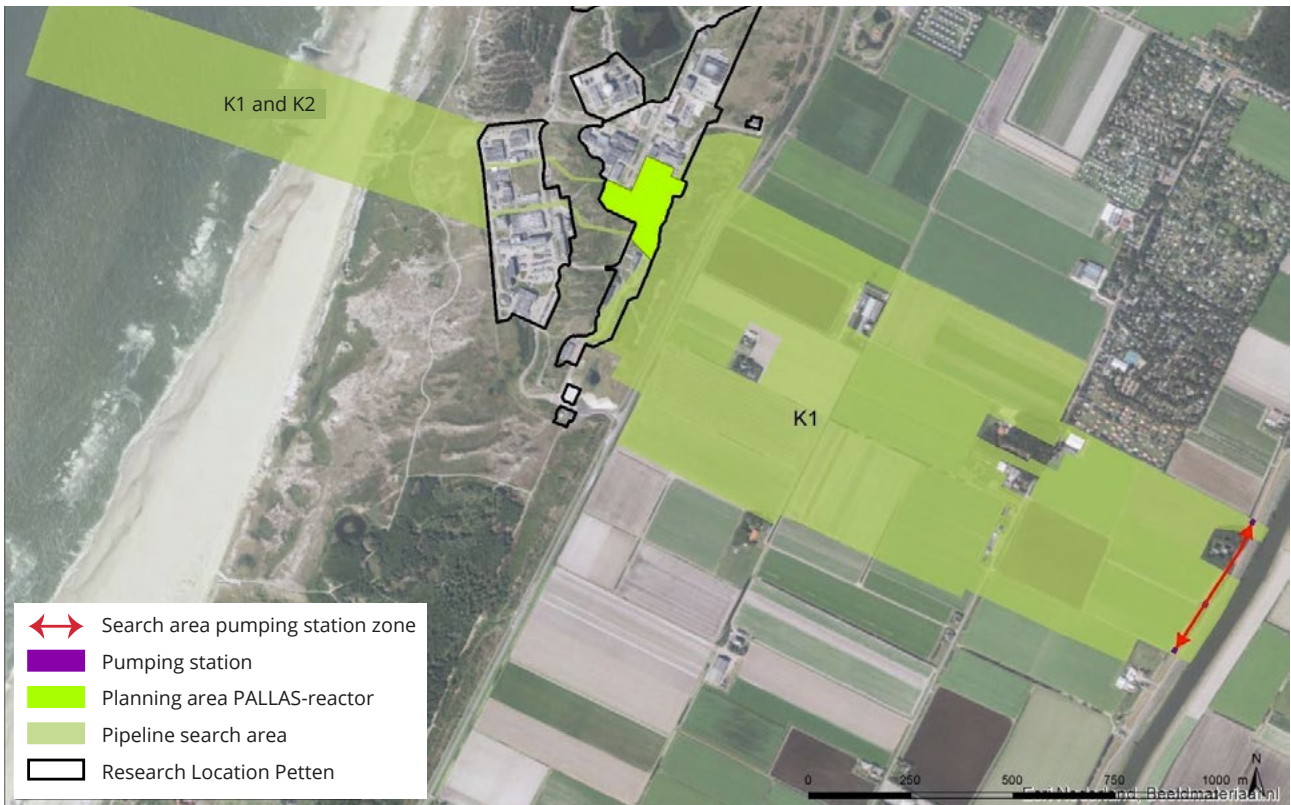
Figure 14 Search area cooling water pipe route and intended new location of new reactor (green shaded area)
